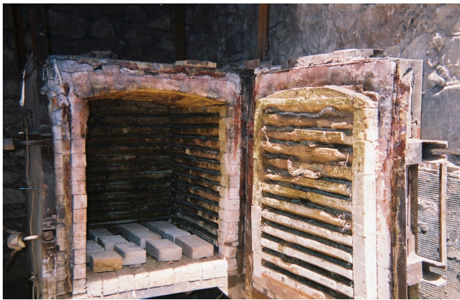
Figure 6 Interior Furnace details
