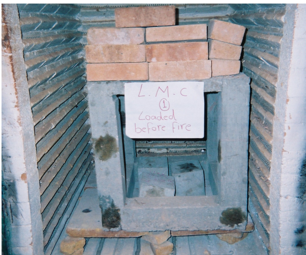
Figure 8 Loaded specimen with cubes prior to heating
